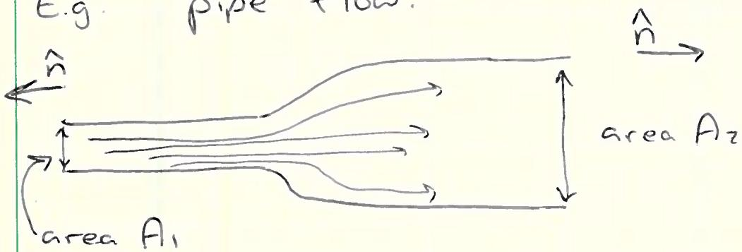
$$0 = -V_1 A_1 + V_2 A_2 \Rightarrow V_1 A_1 = V_2 A_2$$
